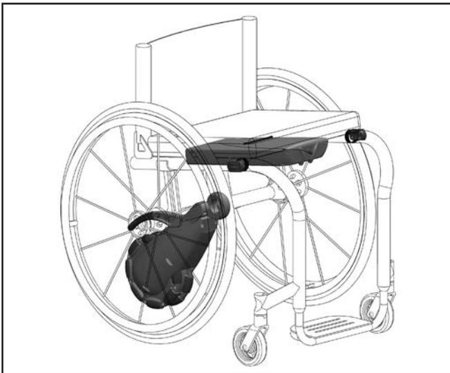
3. Slide the battery back as far back as possible by pushing on the front of the unit. Then plug the button plug into the jack on the front of the battery.
